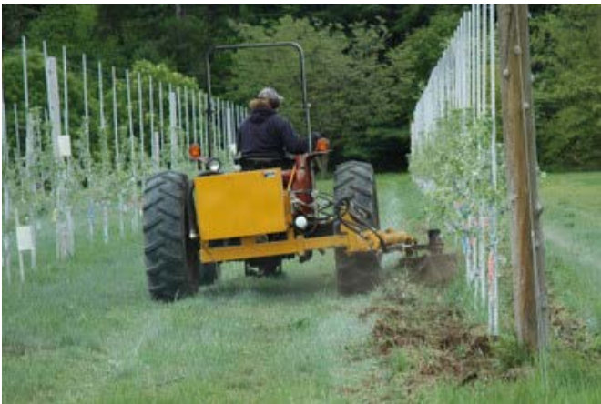
Figure 5. Hydraulic rotary cultivator (Weed Badger™, Marion, ND).
