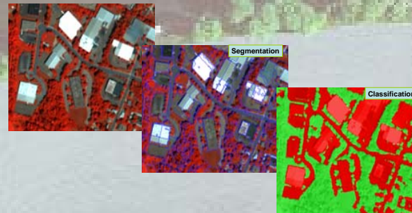
Figure 2. Object-oriented classification of impervious surfaces involves segmentation of pixel reflectance into homogeneous objects (i.e. polygons) followed by hierarchical decision rules for classification.
