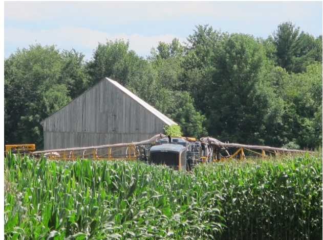
A highboy seeder is used to plant a cover crop in between rows of corn, without damaging or disrupting growth of the plants. Cover cropping is used to limit soil erosion and nutrient runoff, both of which contribute to degraded water quality. (Photo: Northwest Crops and Soils Program)
