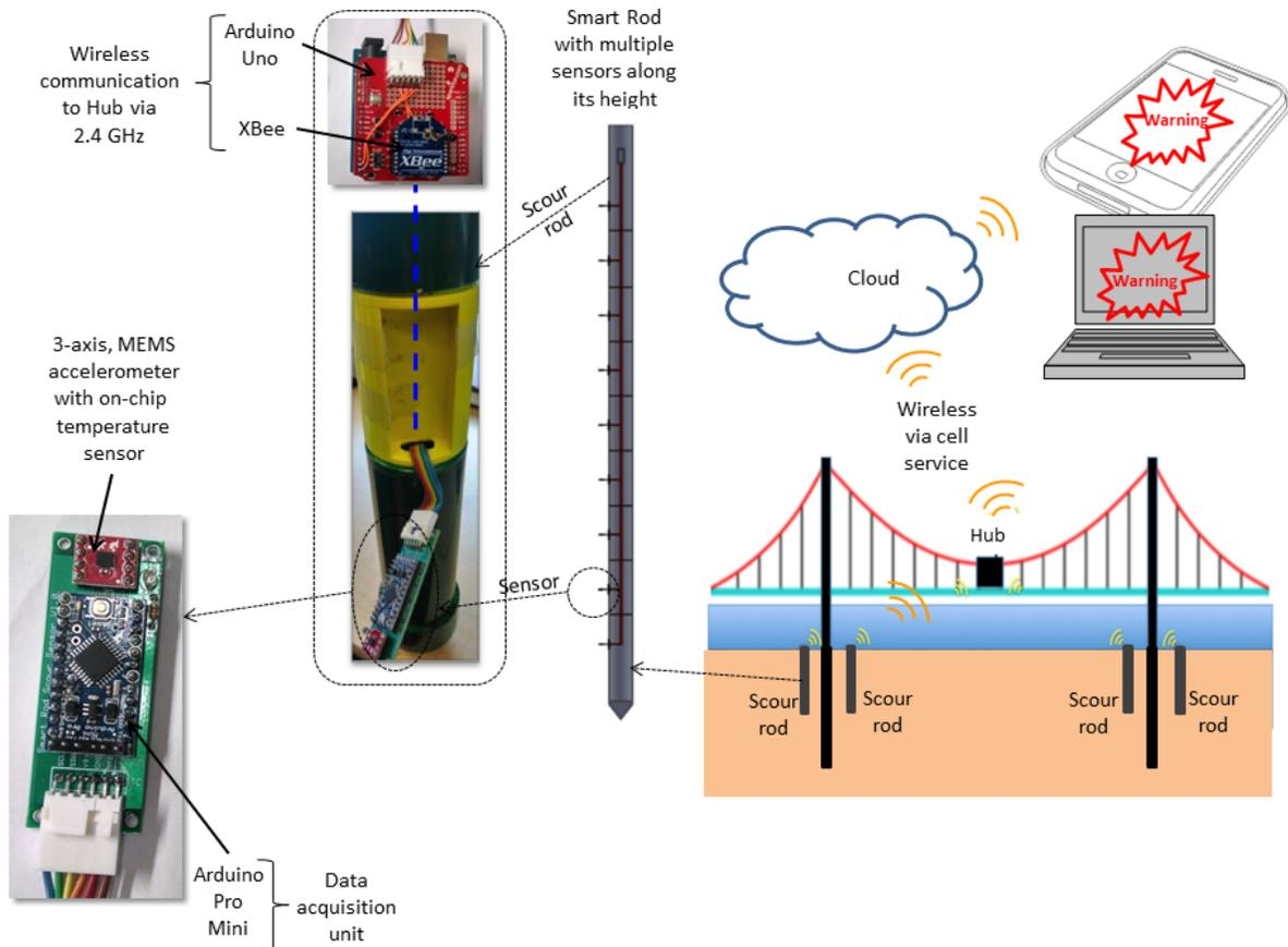
Figure 3.4: Smart Rod scour sensor and communication system
