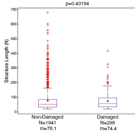
(b) Comparison with respect to the length of the structure
