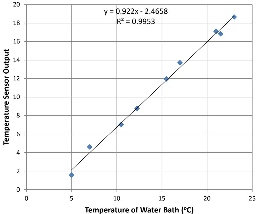
Figure 3.8: Temperature sensor output vs. the temperature
