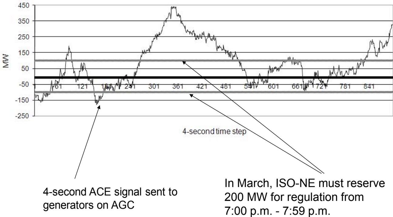
Figure 5-9. Regulation Requirement versus Regulation Use, March 3, 2008 (7:00 p.m.).
