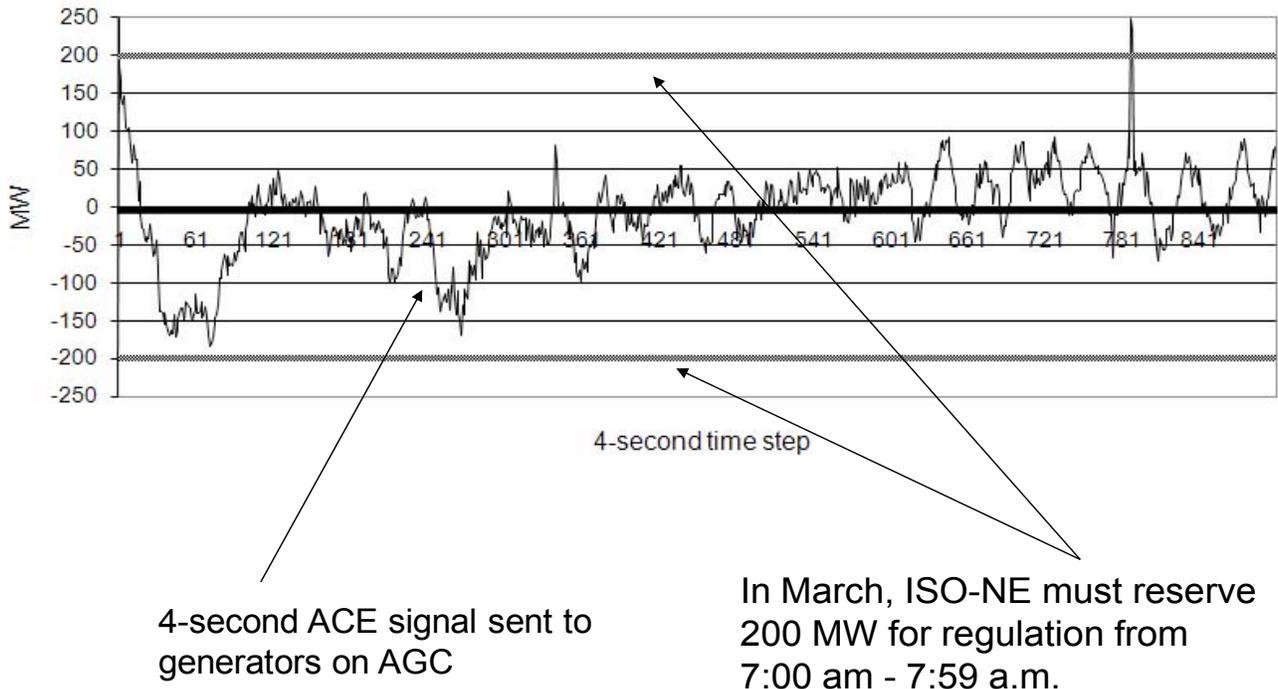
Figure 5-8. Regulation Requirement versus Regulation Use, March 3, 2008 (7:00 a.m.).
