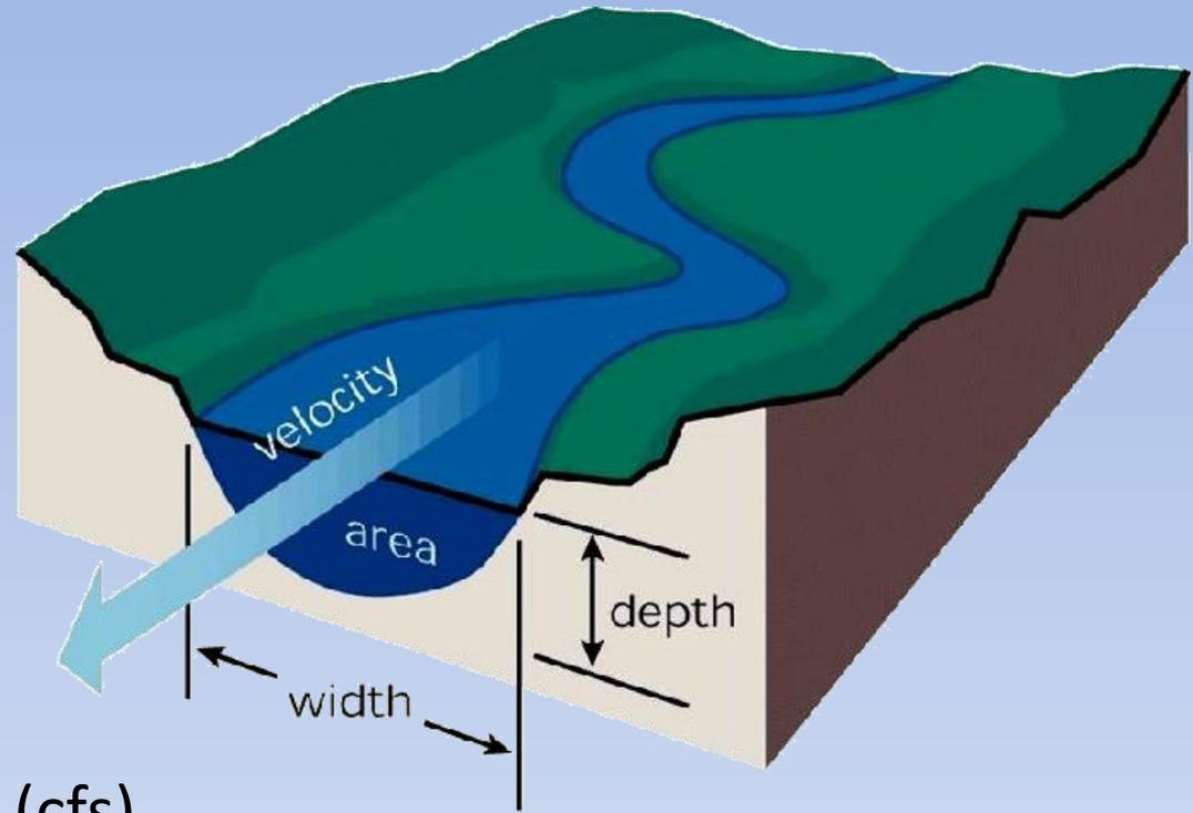
$$Q = v \times A = \text{Discharge (cfs)}$$
