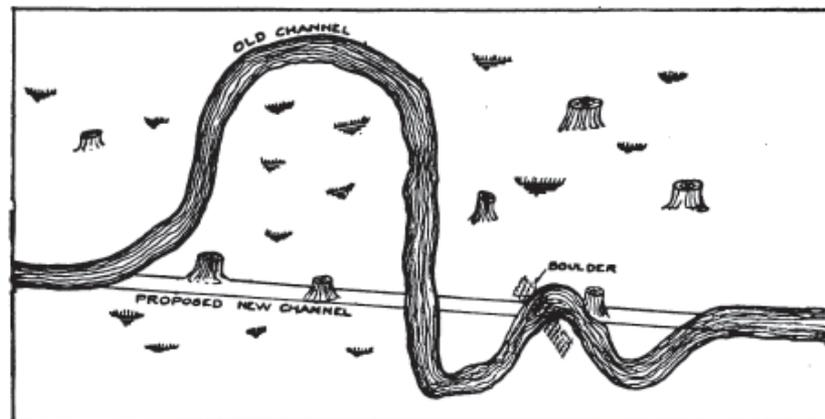
FIG. 54. DIAGRAM OF STREAM TROUBLES THAT MAY BE CORRECTED BY BLASTING.
