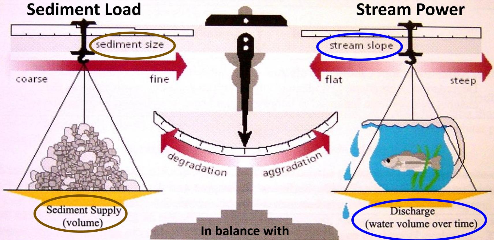
The amount of sediment and the size of the sediment particles that can be transported in a stream are directly related to the gradient (slope) of the stream channel and amount of water flowing in the stream channel at a particular time.
