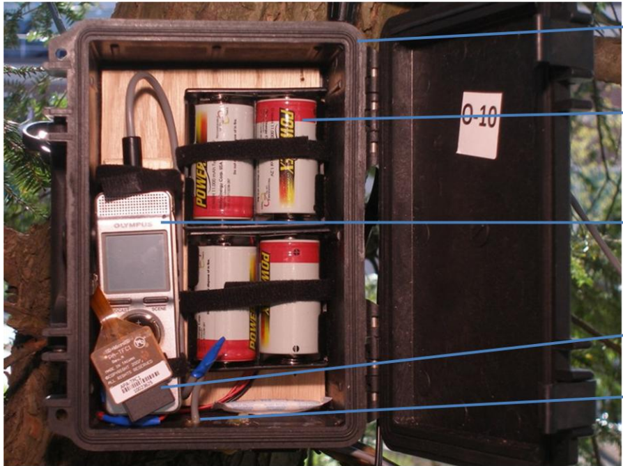
Figure 2. Olympus ARU in the field with front cover open.
