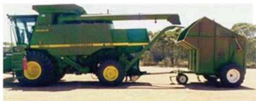
A chaff cart can be towed by the header collecting chaff, straw and weed seeds, thus minimising weed seed return to the seedbank. Photo: Wayne Parker
