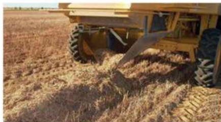
Modifications to the header to generate a narrow chaff trail concentrating weed seeds and allowing a hot burn. Photo: Wayne Parker
