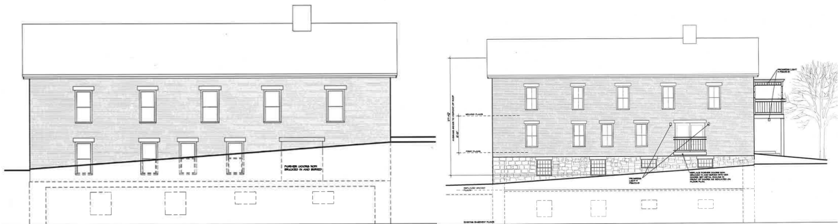
Figure 6. Diagrams of the Existing and Proposed Northern Elevations of the Duncan Blacksmith Shop building, prior to its rehabilitation in 2016. Diagrams from the Historic Preservation Certification Application, Description of Rehabilitation.
