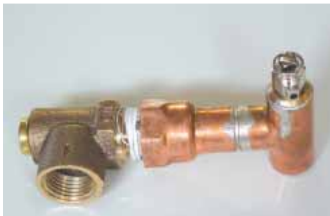
A pressure relief valve and air vent is installed at the highest piping point in the system—the outlet of the solar collector(s).
