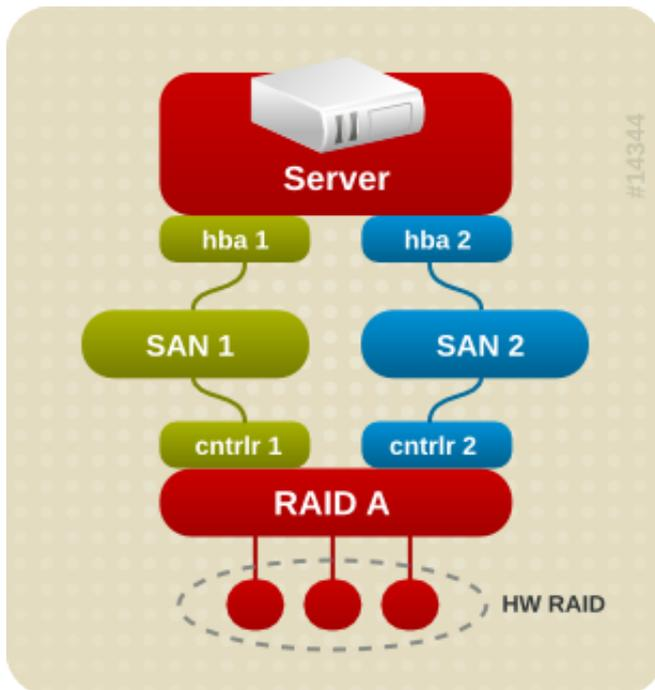
Figure 1.1. Active/Passive Multipath Configuration with One RAID Device
