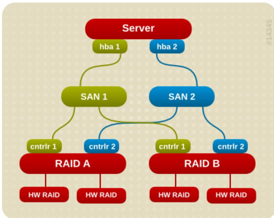
Figure 1.2. Active/Passive Multipath Configuration with Two RAID Devices
