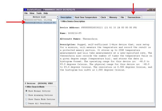
13. Click on the "Thermochron" tab (vertical red arrow above) to program the iButton and to view/download temperature data.
