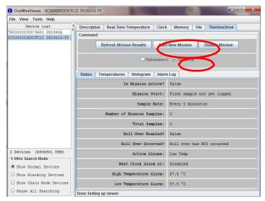
2. As shown below, ENABLE the "Synchronize Real-time Clock" and do **NOT** enable rollover. Enabling this choice on your iButton, once it reaches maximum storage capacity, causes the device to overwrite data from the beginning of the mission and though you are collecting data frequently enough that this shouldn't happen, we don't want you to lose any data. **Be sure that the Sampling Rate is set at 120 minutes (or to sample every 2 hours).**
