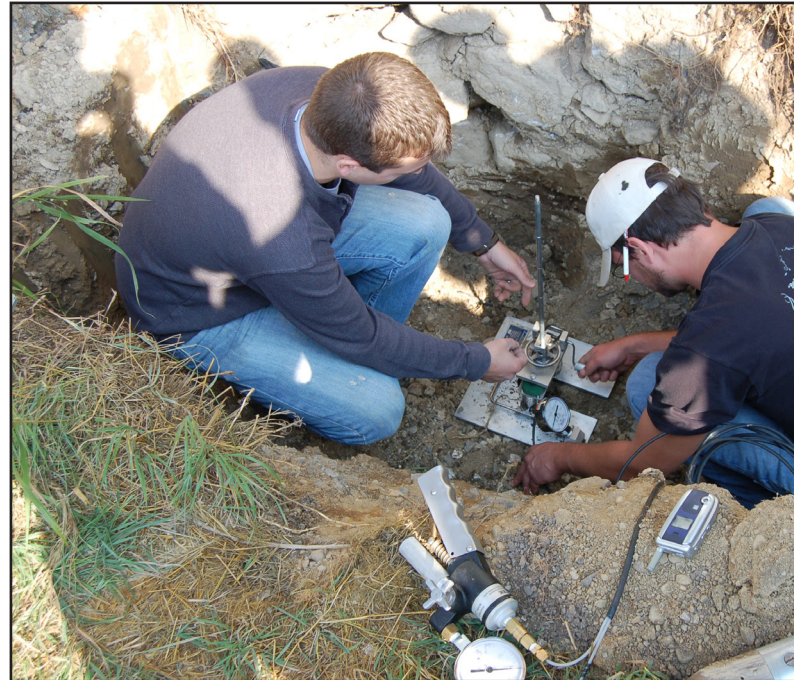
Condition assessment of the barn foundation included test pits for subsurface inspection of foundation stonework, and the collection of geotechnical data.
