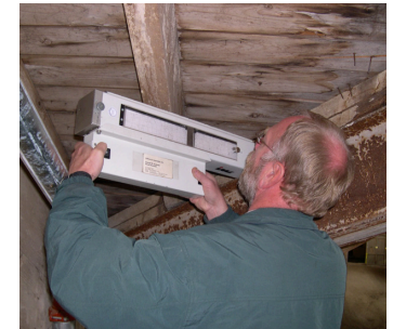
The investigator is using a resistance drill to locate and measure voids in a valley member (top). Note the steel channels that prevent drilling except at the top and bottom of the member. The sample resistograph strip (bottom) indicates a void about 4½-inches in width near the middle of the member. Graphic presentation of resistance drill results for the valley member at 11.0 South (left). The color-coding indicates levels of damage.
