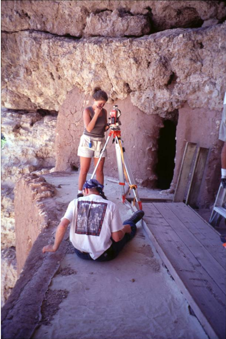
Fig. 2: An upper level terrace at Montezuma's Castle, a National Historic Landmark in Arizona, being recorded with a Total Station Theodolite to connect hand-drawn and photogrammetric data in this 14 th century Sinaguan dwelling. The Texas A&M University team included graduate students in architecture and civil engineering. Photograph by the author, 2002.
