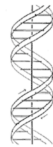
Figure 1. This figure is purely diagrammatic. The two ribbons symbolize the two phosphate-sugar chains, and the horizontal rods the pairs of bases holding the chains together. The vertical line marks the fibre axis.
