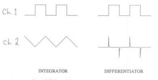
T = 1/150Hz = 6.6msRC = 2X10<sup>4</sup>(10X10<sup>-6</sup>) = 200ms RC >> T  $\begin{array}{l} T = 1/100 Hz = 10 ms \\ RC = 10^6 (295 X 10^{-12}) = .3 ms \\ RC < < T \end{array}$
