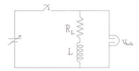
When the switch is closed the bulb is in parallel with the power supply, which is at too low a voltage to cause the bulb to glow. However, the inductor stores energy in a magnetic field. When the switch is opened the following equation applies:
