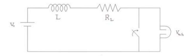
When the switch is closed the bulb is shorted so no voltage builds up across it. However, the inductor stores energy in a magnetic field. When the switch is opened the following equation applies:
