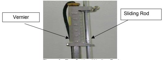
Figure 3. Top-Setting Wading Rod
