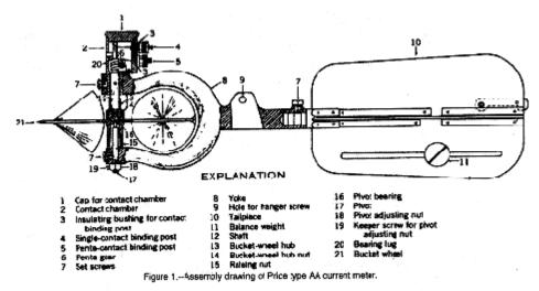
Figure 4. Assembly drawing of Price Type AA current meter
