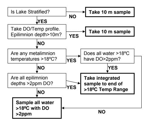
Figure 1. Method for determination of depth-integrated sample for lake water-quality samples
