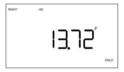
The large number in the center of the display is the distance to the target.
