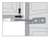
2. To lower a refrigerator door turn the screw clockwise.
