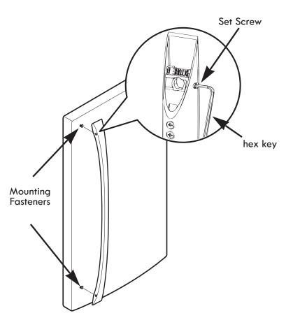
**NOTE:** Removing the doors is always recommended when it is necessary to move the refrigerator through a narrow opening. If it is necessary to remove the handles, follow the directions below.
