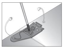
**3.** Using a large phillips screwdriver, turn top hinge fastener counterclockwise to remove the top hinge plate.
