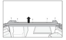
2. Using a large phillips screwdriver, turn top hinge fastener counterclockwise to remove the top hinge/ plate.
