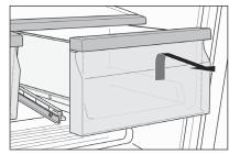
**3.** To install, slightly tilt up the front, insert the drawer into the frame and push it back into place.
