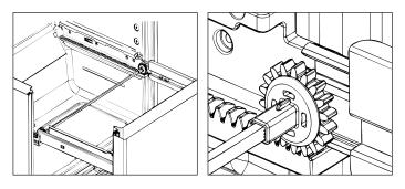
2. Fully push in and close freezer drawer to engage rails with rail support locking tab, applying a bit of pressure after the door is closed to seat the tabs to the rail.
