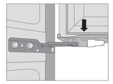
Fit the top hinge over the mounting holes and align to proper position before tightening. Turn top hinge fastener clockwise to secure the hinge.
