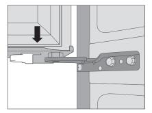
2. Fit the top hinge over the mounting holes and align to proper position before tightening. Turn top hinge screw clockwise to secure the hinge. Insert the ground wire screw and tighten the ground wire (green with yellow stripe) securely beneath it. Reconnect the main wire harness (blue and yellow wires).
