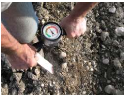
A penetrometer measures compaction in pounds per square inch of pressure. If it takes more than 300 psi to push through a compacted layer, it is unlikely that crop roots will be able to grow through the layer.
