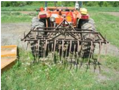
This old Ferguson tine weeder is used for stale bedding fields prior to planting and for blind cultivation over crops like corn while they are still small.
