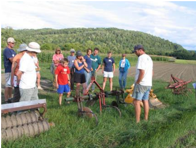
Geo Honigford describes his tillage and cultivation tools at an on-farm workshop. From left to right: cultipacker, 2-row hilling disk set up, rotovator, and an old Ferguson row crop cultivator with C-shanks and shovels.
