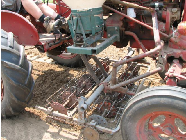
Budding baskets belly mounted on an old IH 140 tractor are used to incorporate pre-plant fertilizer into beds and for stale seedbed control of small weeds before planting crops.
