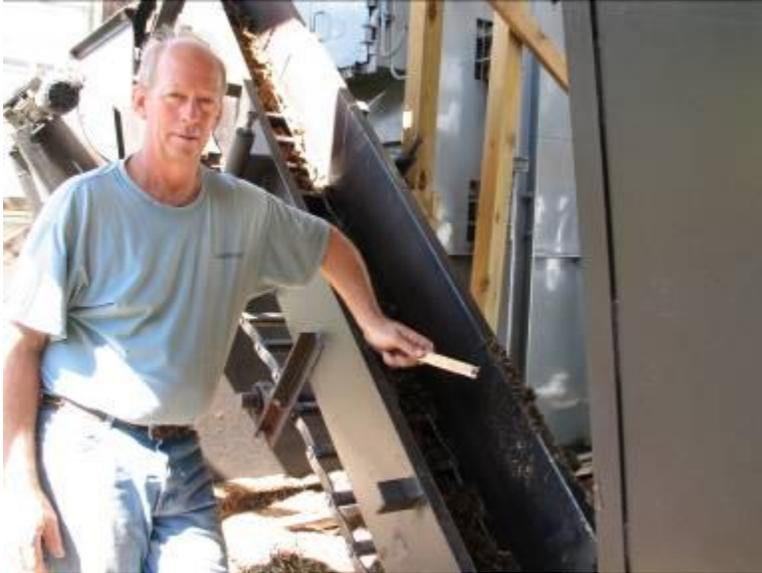
*Fred holds the type of long wood chip that used to cause 'bridging' on his roller delivery system. Now that he uses metal rails to move chips this is less of a problem.*
