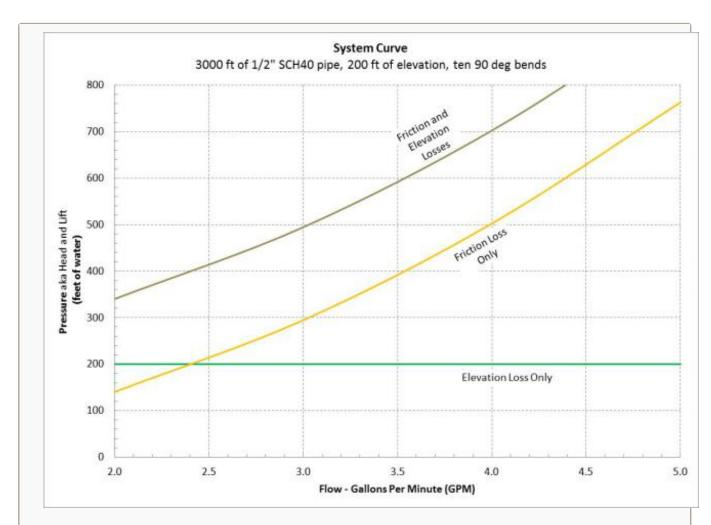
This chart shows the base pressure head required to overcome 200 feet of elevation, but also shows the pressure loss due to 3000 feet of piping and bends. The top line is the total pressure loss as a function of flow for the combination of elevation change and piping losses. Note how this line is curved, not straight. The more flow sent through a piping system the greater pressure loss; or to send more flow through a given piping system the pump will need to generate greater head pressure.
