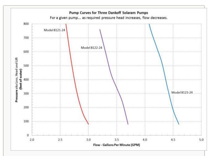
For a given pump, flow depends on the pressure drop of the system. The three pumps noted above are designed for three generally different ranges of flow rates. As pressure head (or piping loss) is increased, the pump provides less flow.
