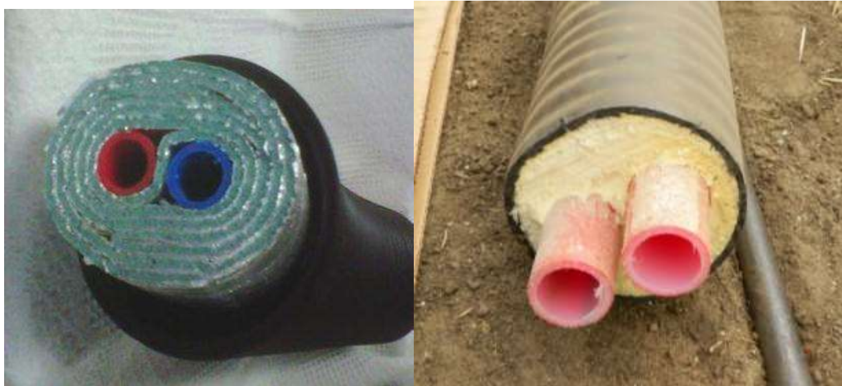
Figure 1 –A less expensive underground insulated PEX tubing option (left) is wrapped in foiled bubble wrap and has space between the insulation on the pipe as well as the outer wall. Cost is approximately $7.00/ft. The solid EPS insulated PEX tube (right) is more expensive at $11.00/ft but has demonstrated reduced heat loss and pipe to pipe heat transfer. Water infiltration is a concern on the foil wrapped version on the left due to the open area that exists.
