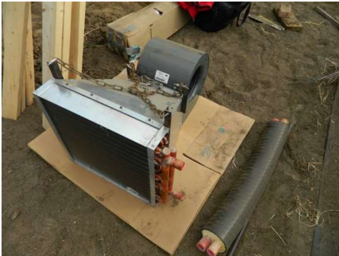
Figure 3 - Air heaters are used to convert the hot water to hot air for space heating in the greenhouse. They consist of a radiator and a fan (left). On the right side of this photo the insulated supply/return PEX can also be seen. This was used for longer runs underground from the boiler to the north house and from the north house to the south house.
