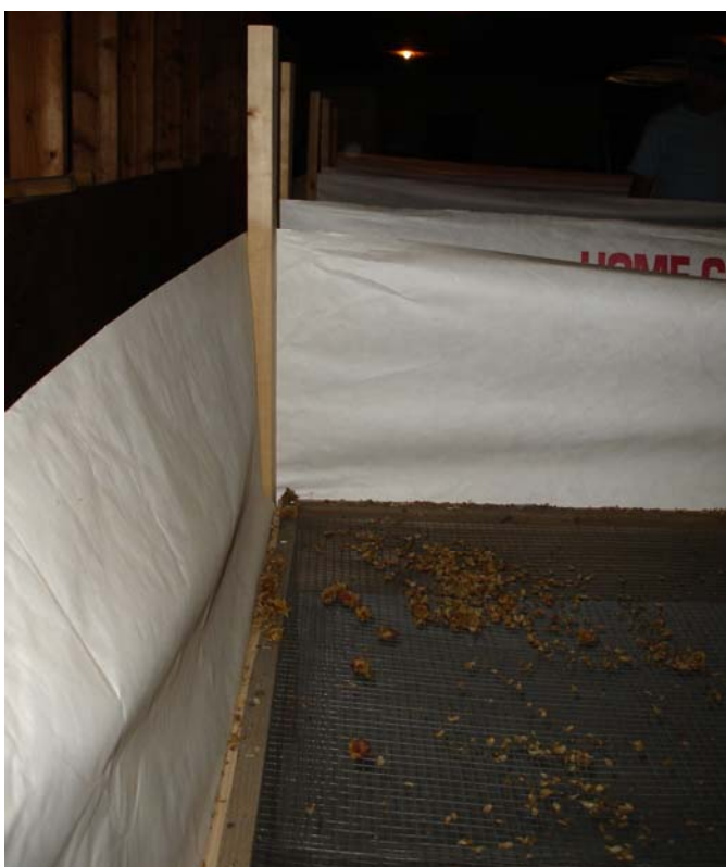
Inside of a home made oast, note the mesh screen installed partway up to allow air to circulate below and above the hops. Note the series of oasts in the background, enabling more volume to be drying simultaneously. Picture of Gene L'Etoile's Four Star Farms, MA. Photo credit r.wilson
