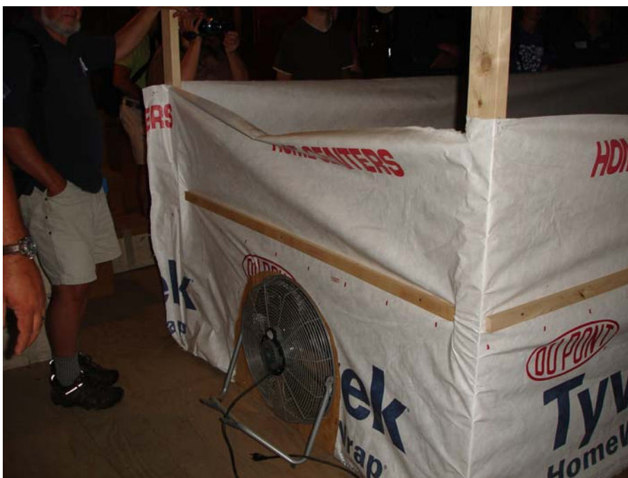
Exterior view of a home made oast. Supplies are simple 2x4's to create the frame, 1x2's to affix the screen, a 4'x8' screen, tyvek to form the walls, and a circular fan. Picture of Gene L'Etoile's Four Star Farms, MA. Photo credit r.wilson
