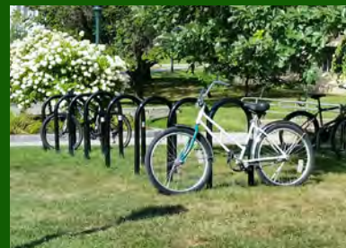
Inverted U-Racks are a superior rack type from a security stand-point, and also better organize bicycles, making them more aesthetically appealing. Inverted U-Racks should become the standard for rack installations across campus
