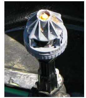
Figure 2. Sprinkler nozzle used in pod.
