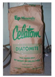
Fig 11: 50 pound bag of diatomaceous earth (DE). For this vendor designation FW-14 works well for filtering vegetable oil
