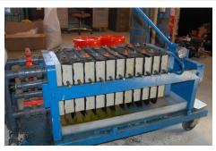
Fig 7: Filter press; a series of filtering plates are pressed together by manual screw or hydraulic pressure.
