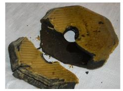
Fig. 8: Block of foots collected from between two filter press plates. The yellowish colored material is filtering media coating (diatomaceous earth) initially placed on filter plate cloth while the dark colored materials are the foots
