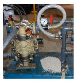
Fig. 9: Air operated diaphragm pump on filter press
