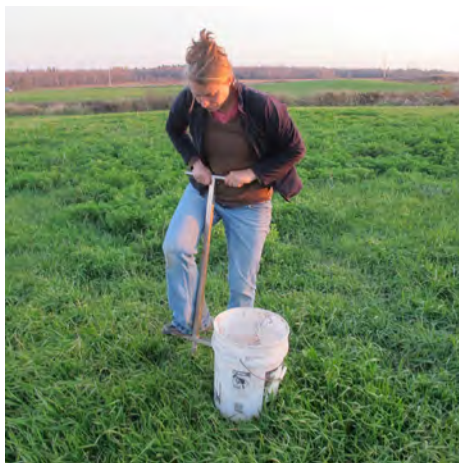
Using a soil probe is the easiest way to get a good soil sample.
