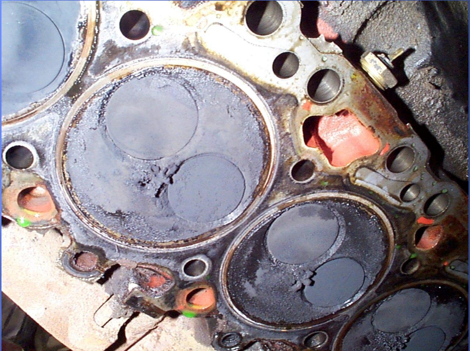
Engine deposit buildups after running on straight soybean oil
