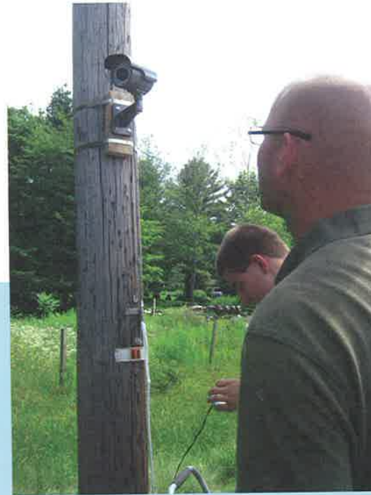
UVM TRC Researcher Jim Sullivan and undergraduate student Ben Rouleau mount a motion activated camera on a utility pole in Williston, Vermont as part of a research project to count bike and pedestrian traffic in Chittenden County.
