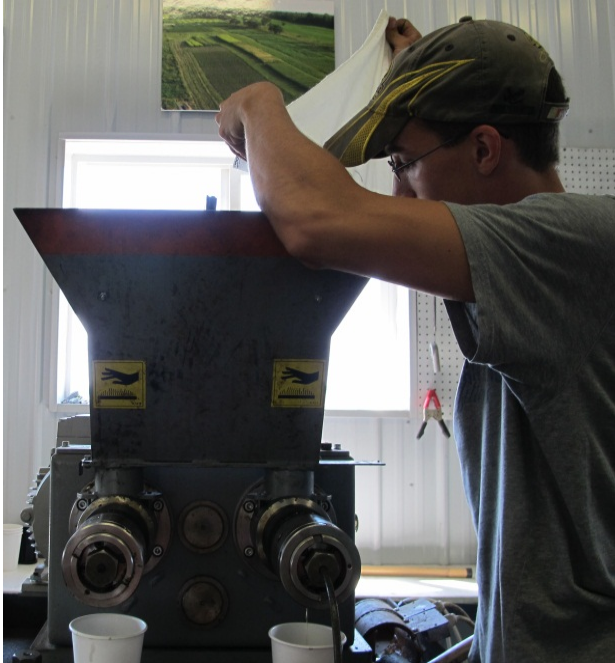
Figure 2. Kern Kraft KK40 press.
