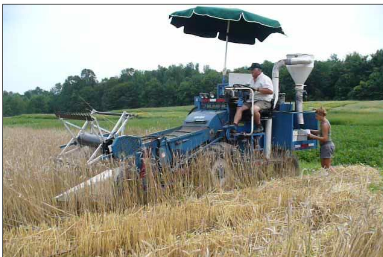
Image 2. Wheat harvest with the Almaco SP50 small plot combine.
