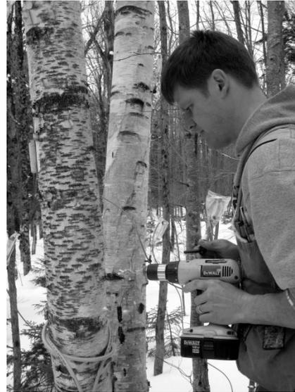
**Researcher Mark Isselhardt of the PMRC prepares a sensor to measure sap pressure in birch.**
