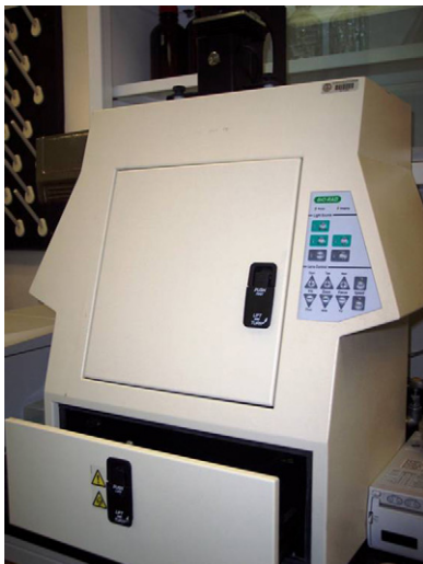
Figure 3. Bioimaging system. UV transilluminators is located inside pullout drawer.
