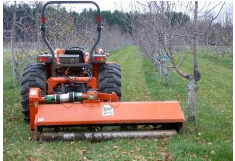
Off-set flail mower used to chop up leaves and winter prunings
