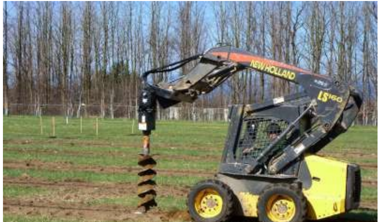
Skid steer-mounted hydraulic auger with 18" diameter bit
