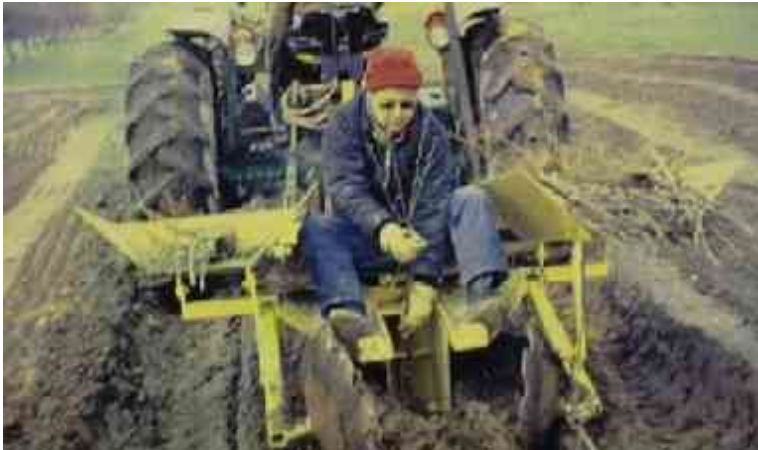
Tractor-pulled tree planter (MSU)
