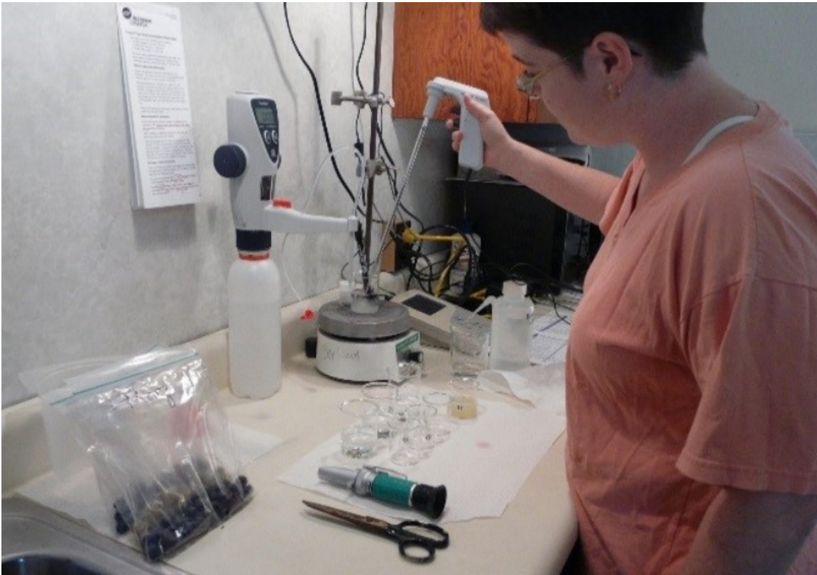
Figure 1: A simple and effective juice field lab can be set up on a bench in the shop, or even on a truck tailgate. Pictured here are (counter clockwise, beginning at lower left): bagged grapes for squeezing; a refractometer for measuring sugars; a pH meter; and a titrator for dispensing NaOH.
