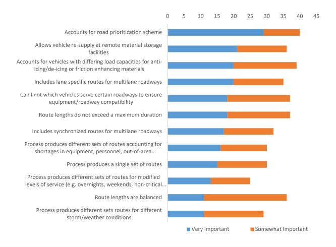
Figure 4.2. Importance ratings for route optimization constraints
