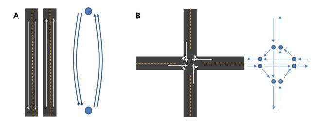
Figure D.3. Network representations (A) allowing lane-specific routing and (B) prohibiting left and U-turns. Modified from Hajibabai et al. (13)
