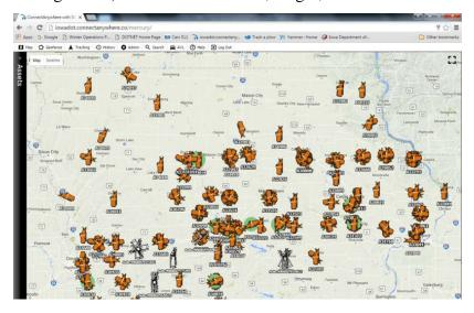
Figure 5.2. Web interface for Iowa DOT's AVL system.
