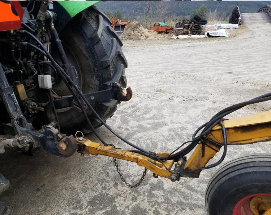
Once the two hydraulic lines are hooked up, lift the unit to relieve tension and remove the transport lock pin in order to lower the drill and put it in field mode.
