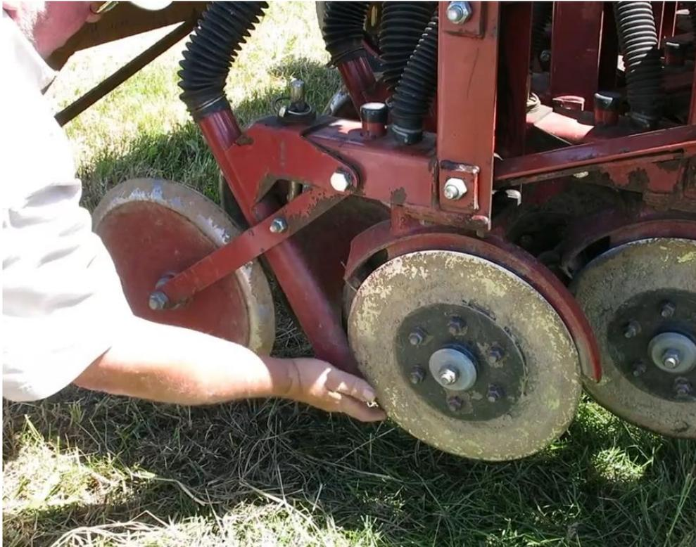
Check all the grease fittings on the unit, and grease if necessary.
