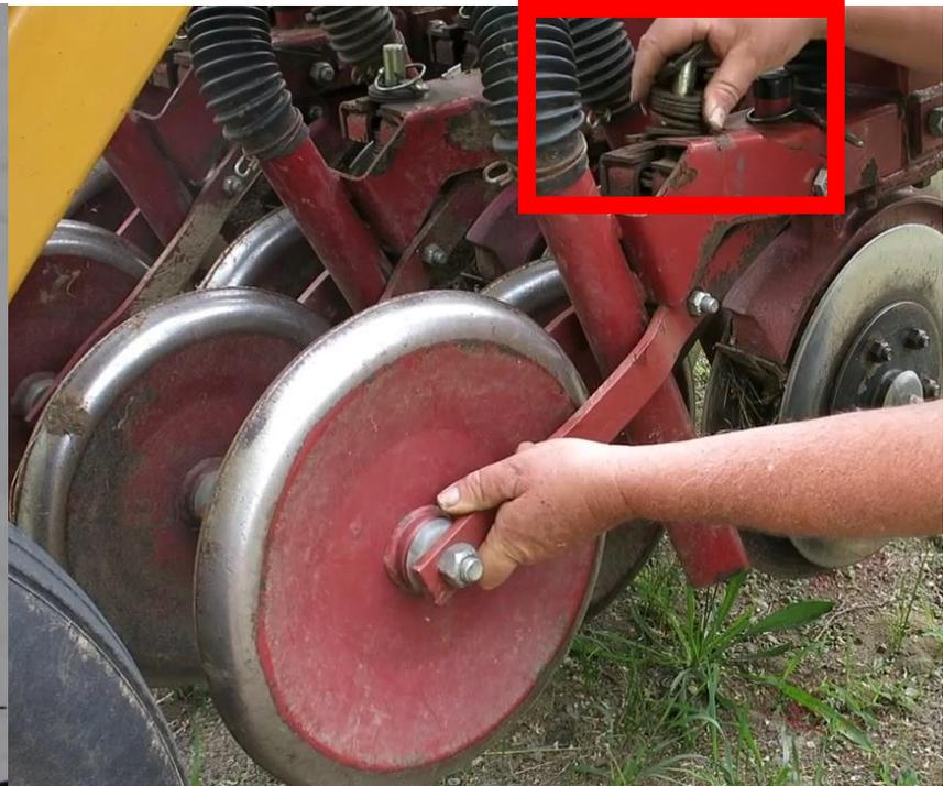
Raise the press wheels by moving washers from the bottom of the pin to the top; to lower them, move washers from top to bottom. Repeat for all press wheels.
