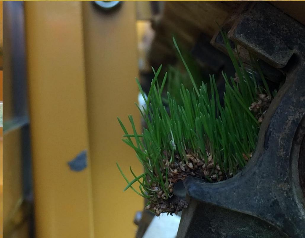
Photos of clogged seed tubes and seed box openings.
