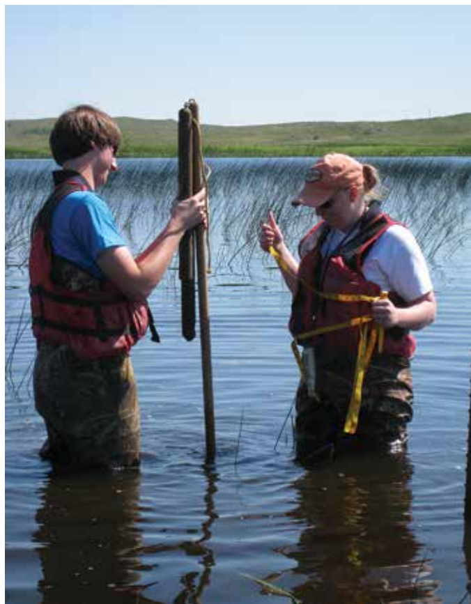
Undergraduate students (Jason Augspurger, left; Donna Abler, right) record substrate firmness in a Nebraska Sandhill lake. Photo credit: Mark Kaemingk.
