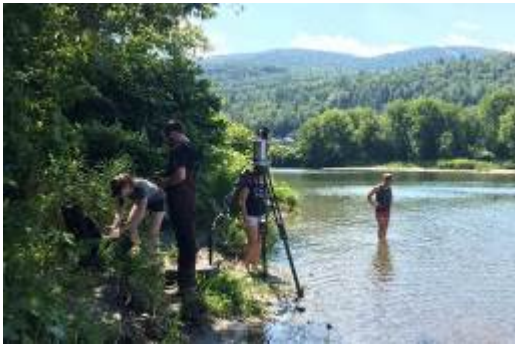
Figure 7. Terrestrial LiDAR data collection along the Winooski River with graduate student Thomas Bryce and undergraduate researchers
