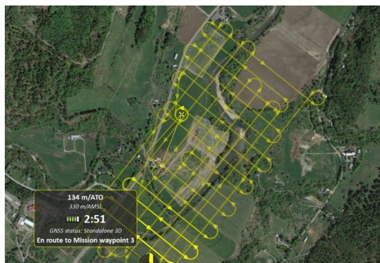
Figure 5. Mapping area along a section of the Mad River covering the MR-B site for a single flight. Yellow lines are user-selected, pre-programmed flight lines that the UAS follows automatically.
