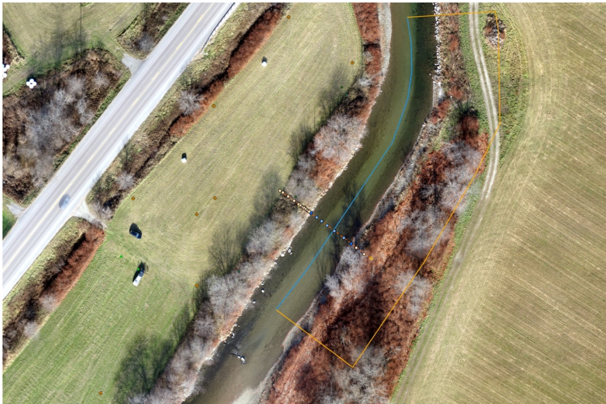
Figure 9. MR-B field site on the Mad River showing UAS imagery, area of terrestrial laser scanning, ground control points and also location of cross section survey with GPS
