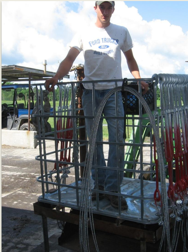
Home made lift bucket. Made from a 250 gallon tote holder
