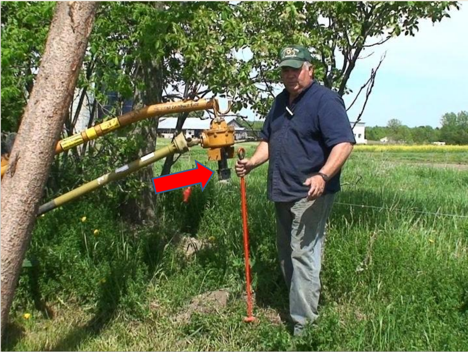
3 Point Hitch Post Hole Digger With Anchor Attachment
