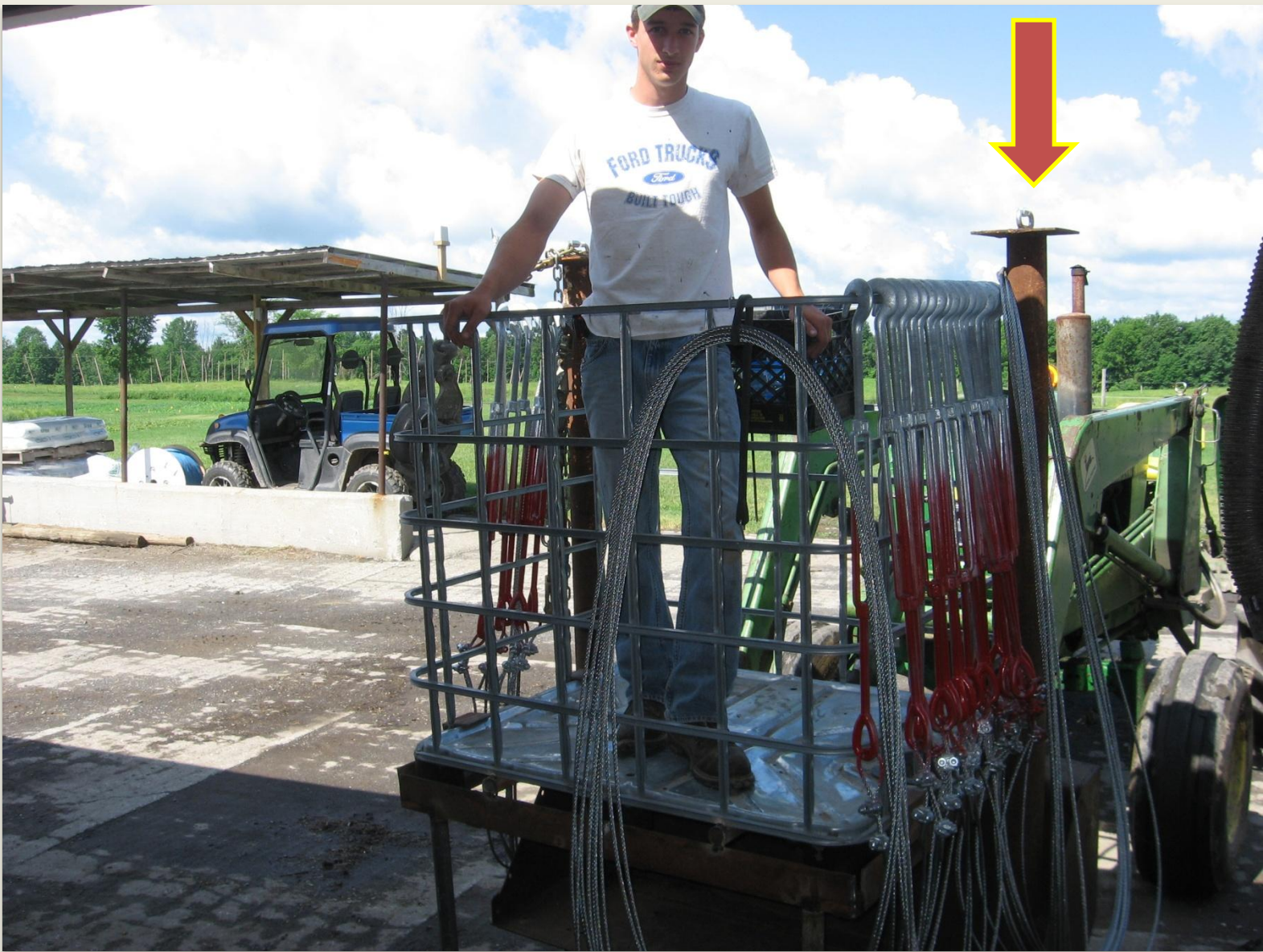
Eye hook for mounting Haven Grip for pulling cable
