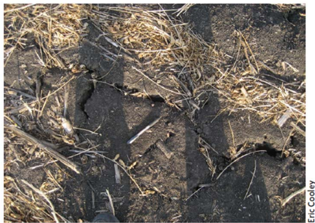
Figure 3: Cracks in clay soils with high shrink-swell capacity.
