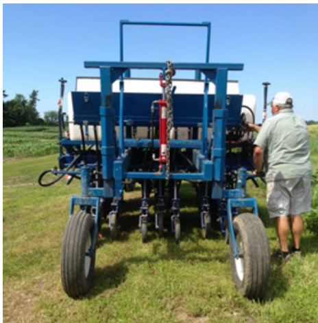
PennState cover crop interseeder and applicator.
