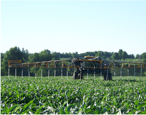
High clearance cover crop interseeders like the “highboy” pictured here can effectively seed cover crops prior to corn harvest. Photo credit: UVM Extension NWCS.
