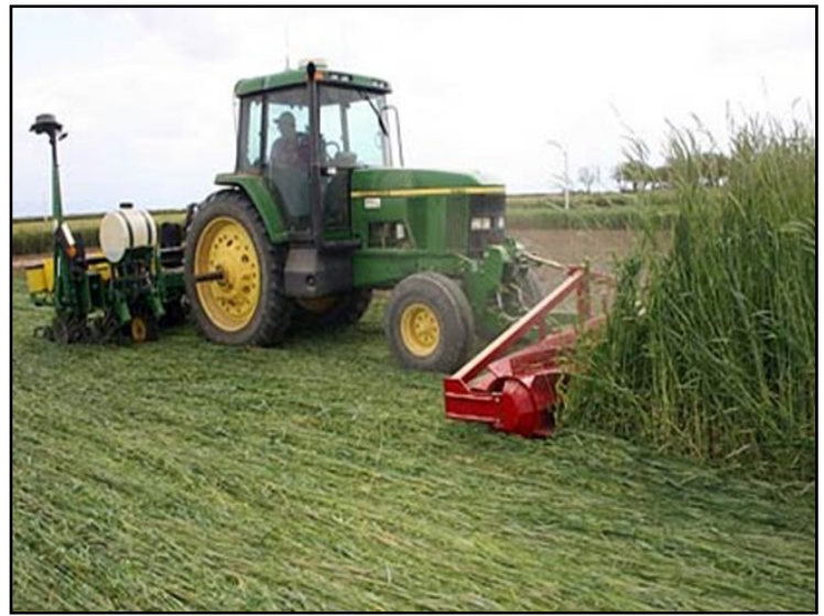
Figure 4. Front mounted Roller Crimper. Source: https://rollercrimpers.com/pictures
