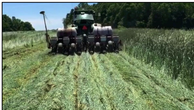
Figure 1. Planter mounted Dawn ZRX Roller Crimper used to roll cereal rye while planting corn crop.
