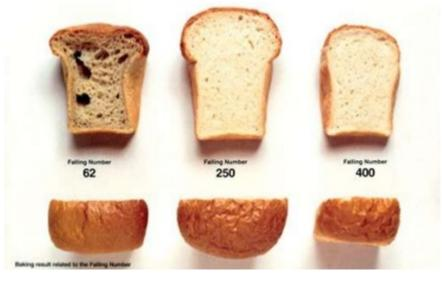
nate. If a falling number is low it means the grain has begun to germinate, enzymatic activity is high, and the plunger falls through the slurry quickly.
